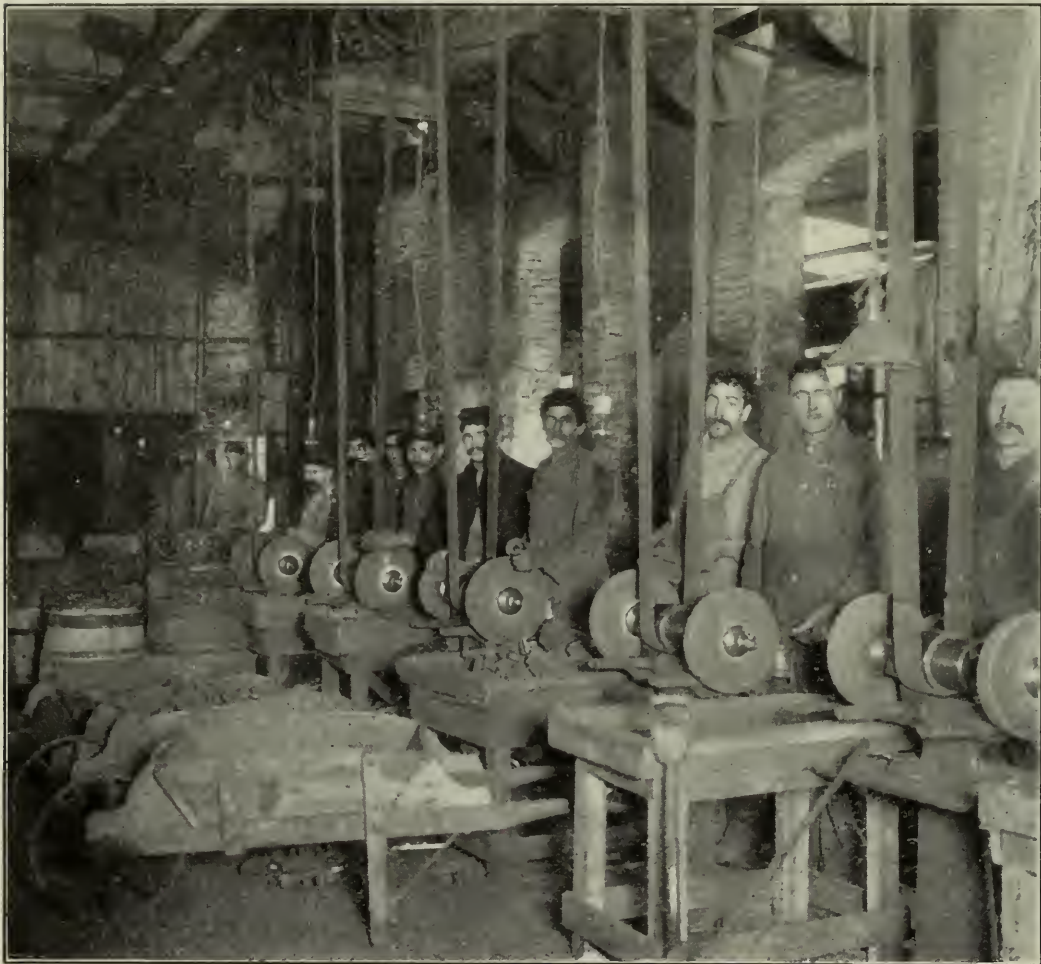
CARBORUNDUM WHEELS IN GRINDING ROOM OF THE WHITINSVILLE MACHINE WORKS, CAST-IRON DEPARTMENT.
